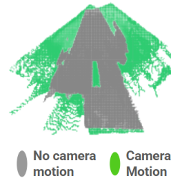
Fig. 4: Voxel coverage with a fixed (gray) vs. panning (green) camera, showing the additional environment coverage gained through camera motion.
